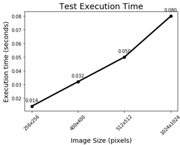
FIGURE 7. Test time comparison between different sizes of test images and their execution time. Increasing the test image size correspondingly increase the test time.
