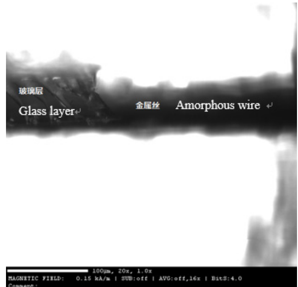
FIGURE 3. Microphotograph of corroded glass coating.
