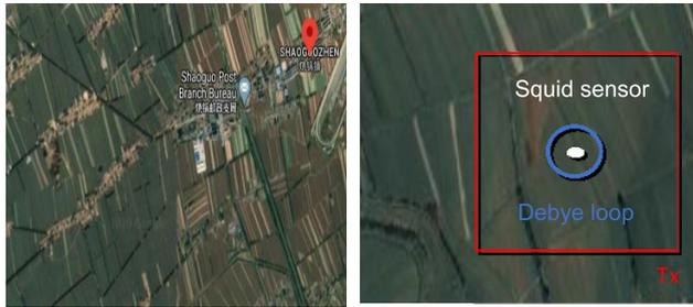
**FIGURE 10.** TEM field measurement in Shaoguo town: (a) location in Google map; (b) TEM devices setting, where red square loop (Tx) is the transmitter loop, the blue circle at the center shows the Debye loop, and the white dot at the center shows squid sensor that can record  $B$  field.
