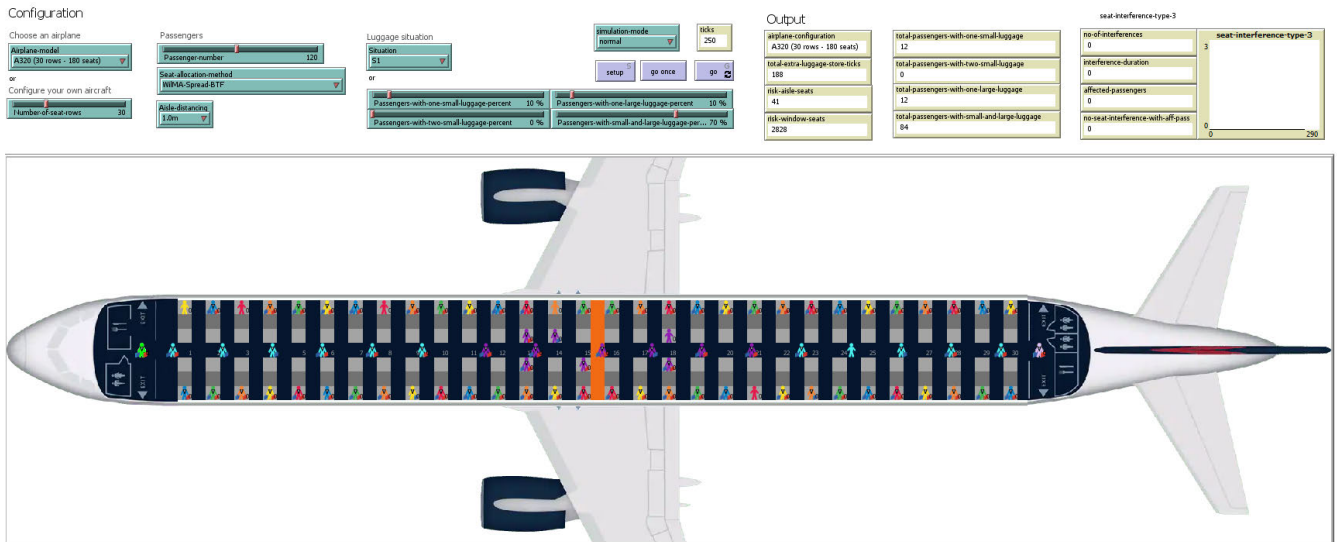
FIGURE 14. The GUI for the agent-based model in NetLogo 6.1.1 (example of view for WilMA-Spread-Back-to-front method with 1 m social distancing).
