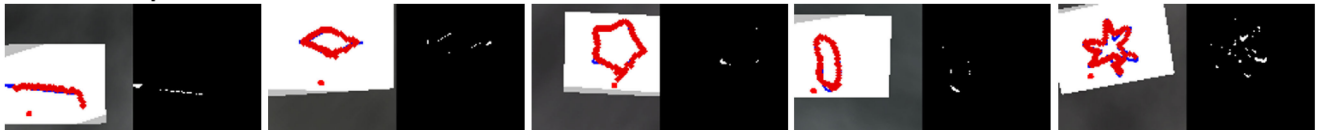
FIGURE 20. Evaluation results on the learned and unlearned target patterns using the SDC policy in a randomized environment. For each pattern, the left image shows the target pattern image and generated path on it. The right image shows the pattern image reduced by the laser pointer path of the left image.
