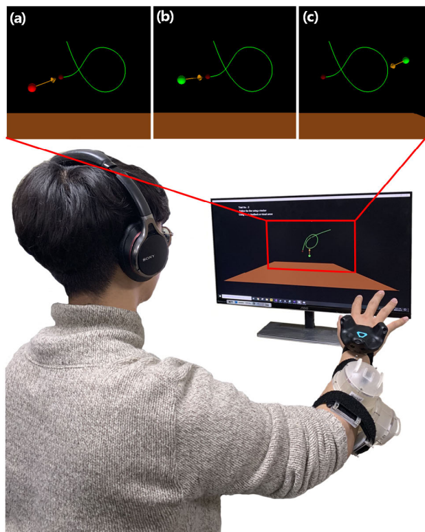
FIGURE 9. Experiment Setup. The participant wore the haptic interface and VIVE tracker to conduct Experiment 1.
