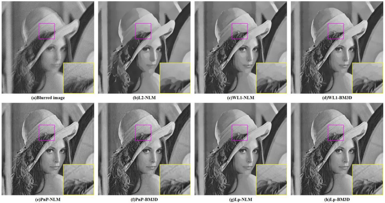
FIGURE 8. Restored results for motion blurred ( L = 5, \theta = 10^\circ ) image Lena by different methods.
