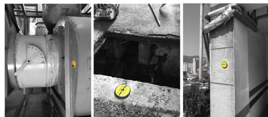
FIGURE 1. Installation of a LoRa device with a vibration detection sensor in various environments. The device is highlighted with a yellow color for easy identification in the photos.
