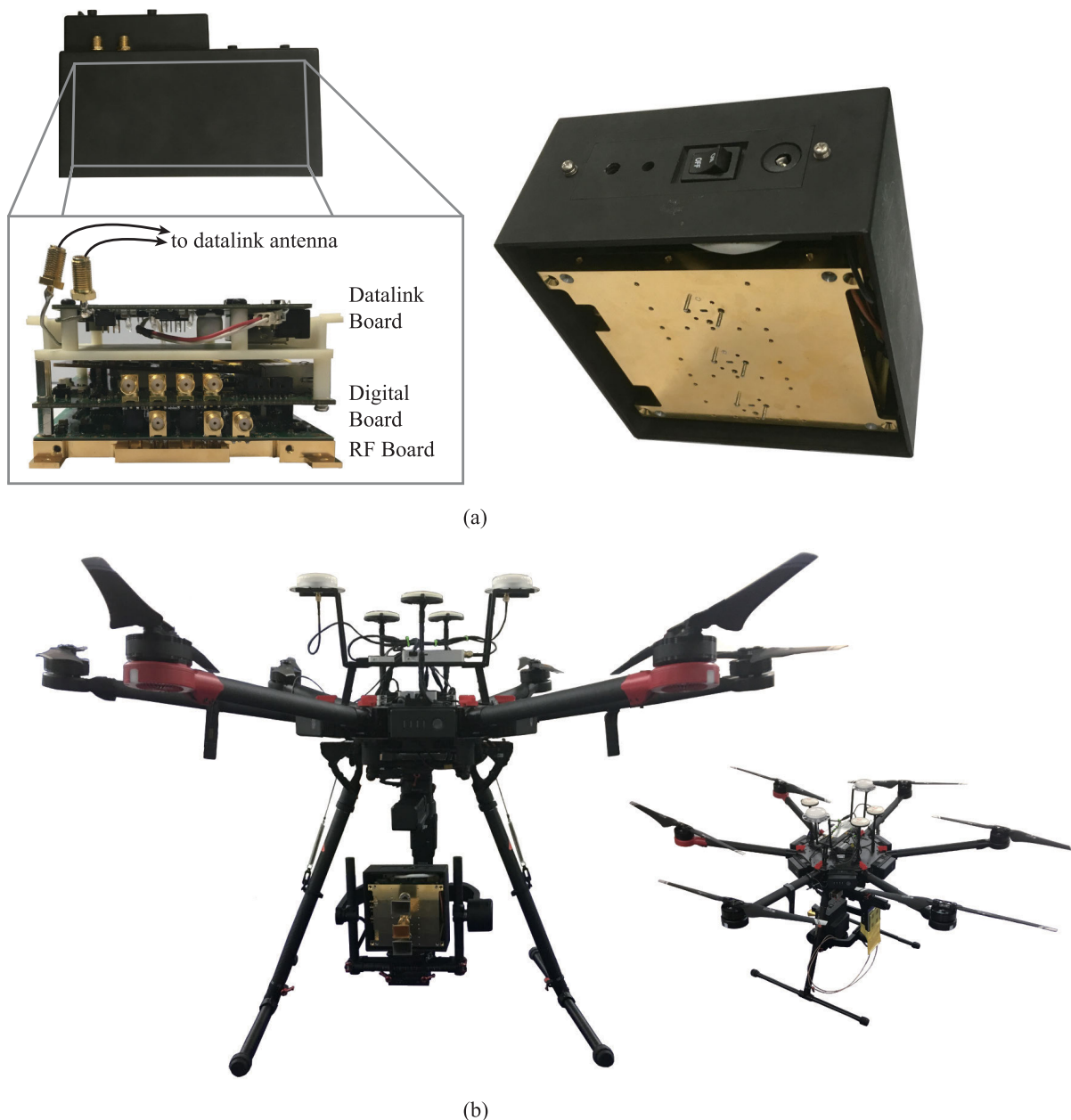
FIGURE 5. Picture of the radar system. Image (a) shows a picture of the plastic case, three stacked boards, and the radar system, and (b) is a picture of the SAR system mounted on the platform.
