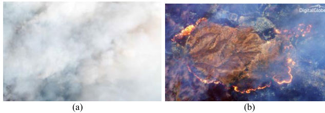
FIGURE 2. Forest fire burning [6]. (a) The visible part of the spectrum – the smoke completely obscures the ground. (b) SWIR image, which made from three of eight SWIR bands – the smoke disappeared and coincidentally give an orange color to the fires.
