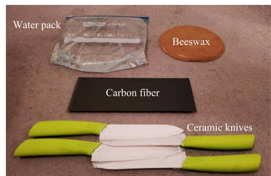
FIGURE 12. The materials that have been measured using the 20 GHz radiometer of Figure 11. From the top: the water pack (left), the yellow beeswax (right), the carbon fiber, and the ceramic. In the case of the ceramic, a larger surface area was created by fixing four (20 cm long bladed) ceramic knives together.
