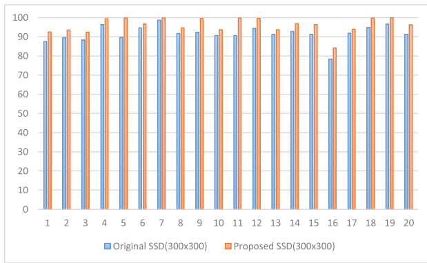
FIGURE 6. A comparison of precision of different models for 20 type of items between the proposed SSD and the original SSD.
