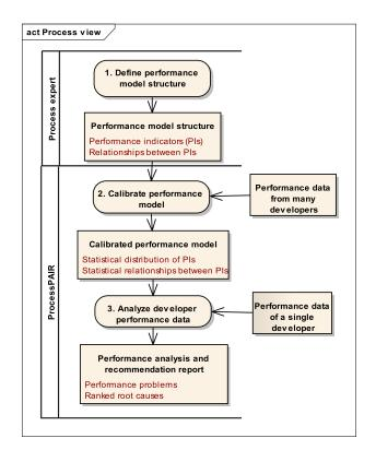
FIGURE 1. UML activity diagram depicting the main activities and artifacts in the ProcessPAIR method.
