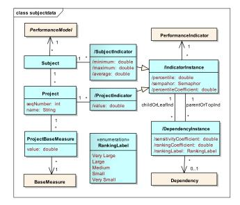
FIGURE 6. UML class diagram depicting the main concepts involved in the analysis of subject data.
