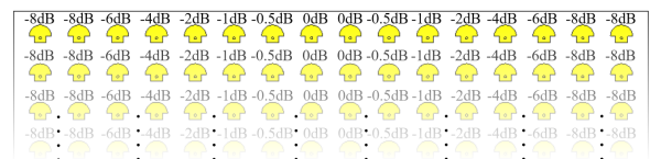
FIGURE 13. The applied rounded amplitudes per antenna element.
