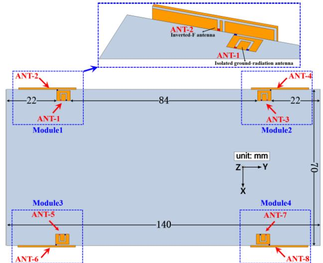
**FIGURE 11.** Antenna configurations of the proposed 8 × 8 MIMO antenna array.
