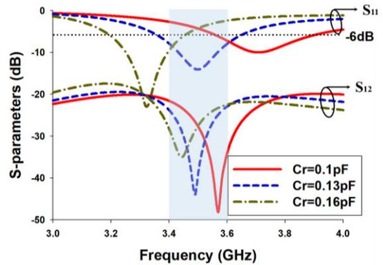
**FIGURE 7.** Simulated S-parameters with the variation of the capacitor value  $C_r$ .
