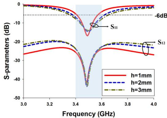
**FIGURE 6.** Simulated S-parameters with the variation of the height  $h$  of the out-of-ground loop.
