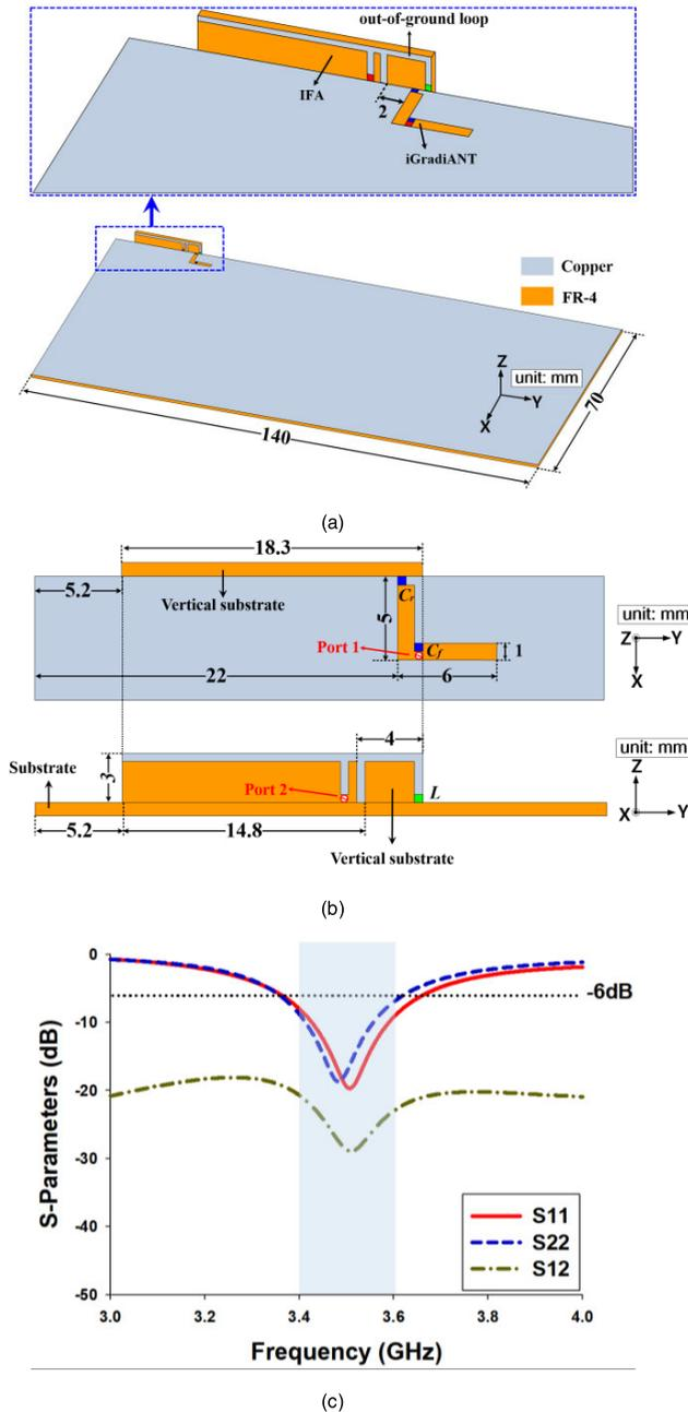
**FIGURE 8.** Antenna configurations of the compact design of the proposed  $2 \times 2$  MIMO antenna set: (a) perspective view, (b) side view, and (c) simulated S-parameters.
