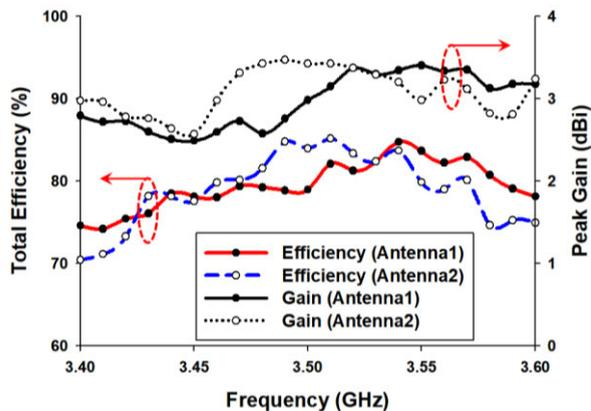
FIGURE 14. Measured total efficiencies and peak gains of the proposed  $8 \times 8$  MIMO antennas.
