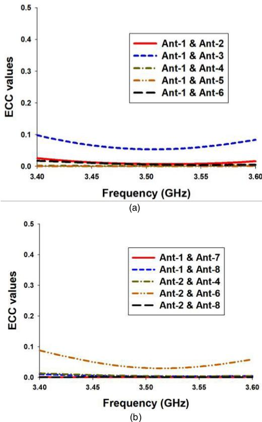
FIGURE 16. Measured ECC values of the proposed 8 × 8 MIMO antenna array.
