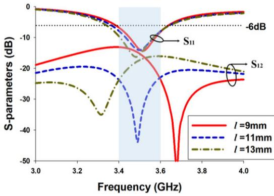
**FIGURE 5.** Simulated S-parameters with the variation of the length  $l$  of the out-of-ground loop.
