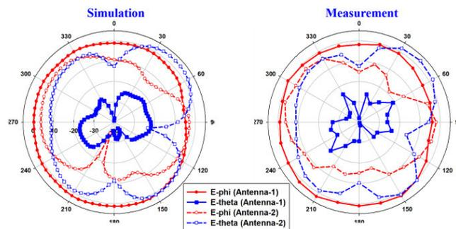
FIGURE 15. Simulated and measured radiation patterns of the proposed  $8 \times 8$  MIMO antenna array in the  $xz$ -plane at 3.5 GHz.
