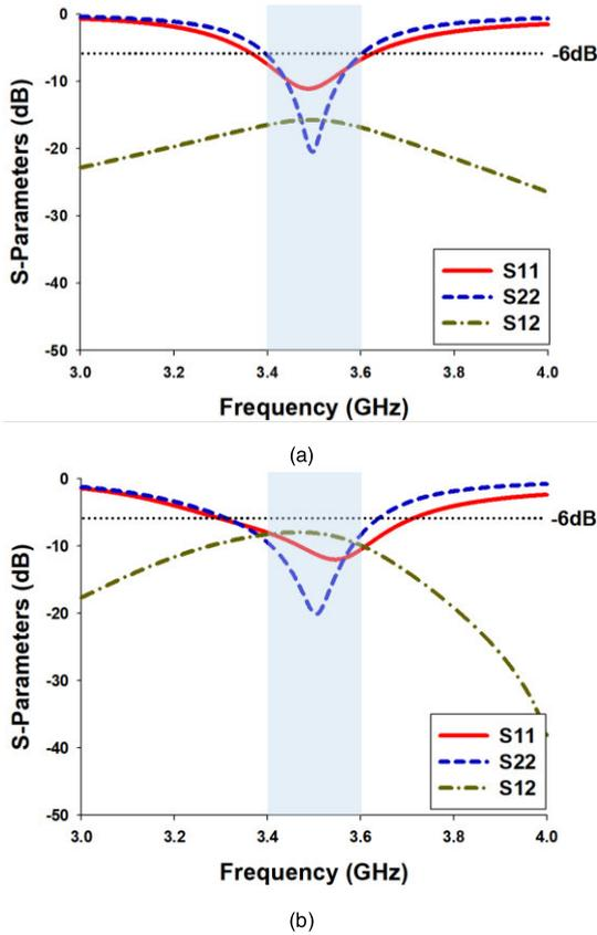
**FIGURE 10.** Simulated S-parameters: (a) Integration of iGradiANT and the loop antenna, and (b) the reference MIMO antenna set (without the out-of-ground loop).
