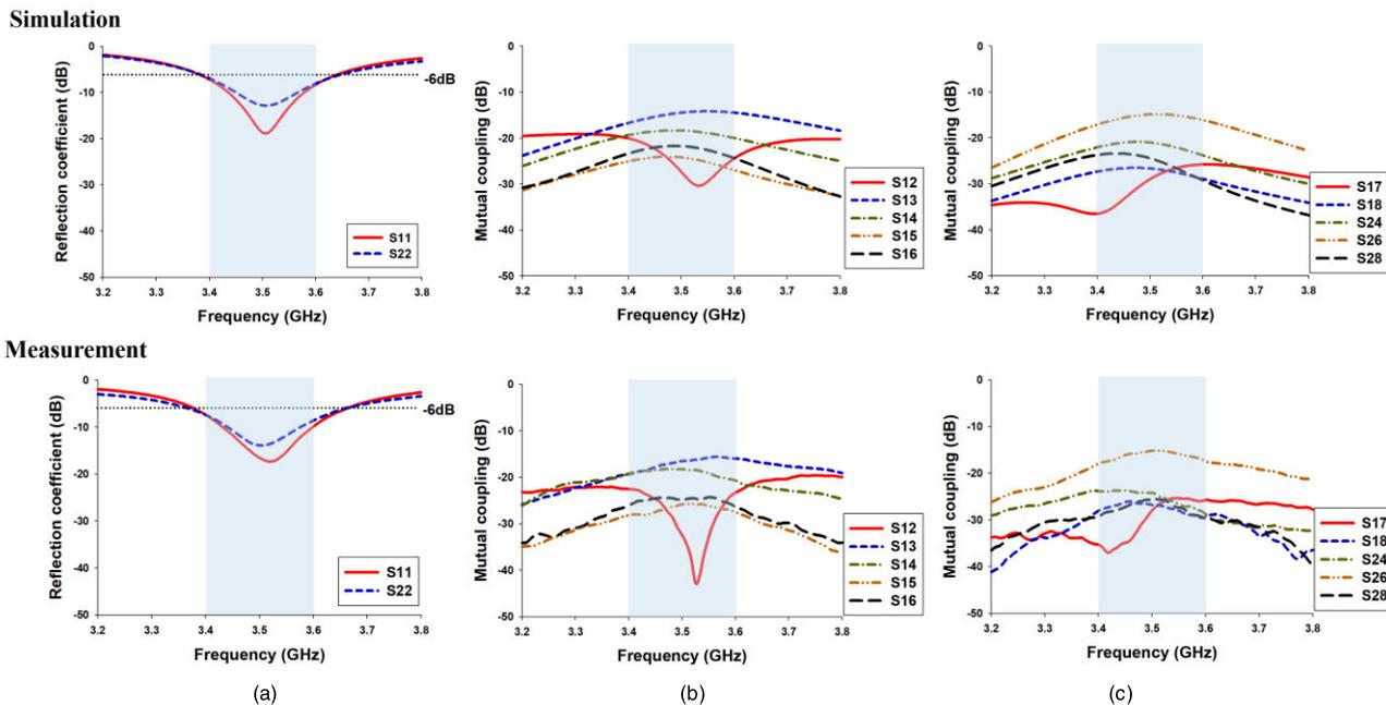
FIGURE 13. Simulated and measured S-parameters of the proposed  $8 \times 8$  MIMO antenna array: (a) reflection coefficients, (b), and (c) mutual coupling.
