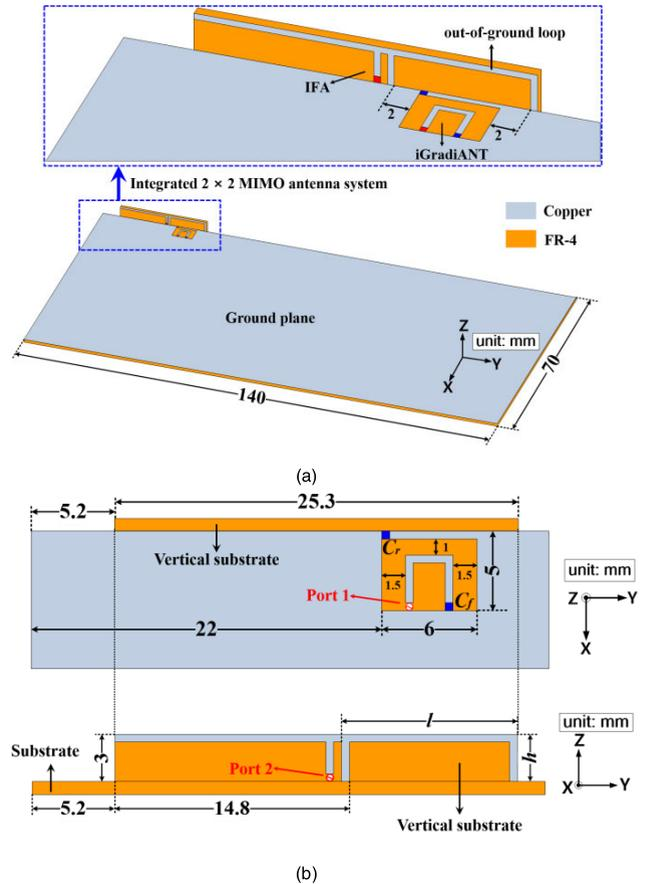
**FIGURE 2.** Antenna configurations of the proposed integrated MIMO antenna set: (a) perspective view, and (b) side view.
