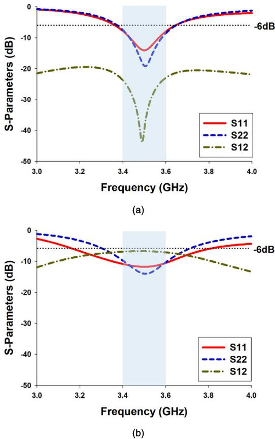
**FIGURE 3.** Simulated S-parameters: (a) the proposed integrated MIMO antenna set, and (b) the reference MIMO antenna set.
