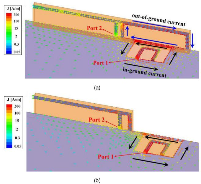
**FIGURE 4.** Simulated surface current distributions: (a) the proposed integrated MIMO antenna set with excitation of the iGradiANT at 3.5 GHz, and (b) the reference MIMO antenna set with excitation of the traditional GradiANT at 3.5 GHz.
