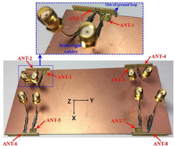
**FIGURE 12.** The prototype of the fabricated 8 × 8 MIMO antennas.
