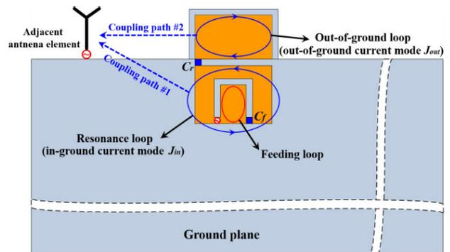
FIGURE 1. Schematic diagram of the iGradiANT for MIMO antennas.
