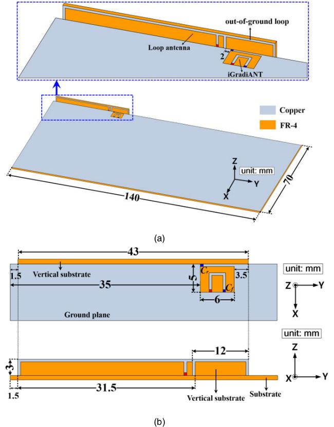
**FIGURE 9.** Integration of iGradiANT and a loop antenna: (a) perspective view, and (b) side view.
