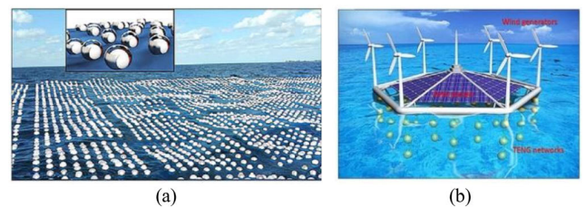
FIGURE 28. Aggregated form of TENG: (a) a spherical ball based TENG network. (b) combined arrangement with other RESs [57], [59].
