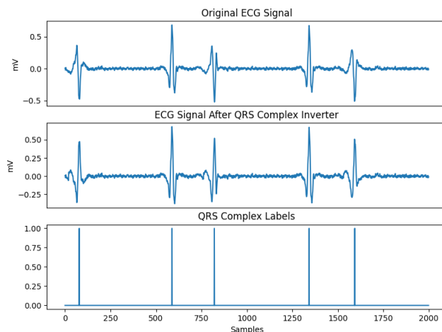
FIGURE 6. QRS complex inverter flipping inverted QRS complexes.
