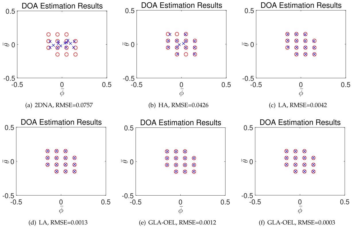
FIGURE 7. The DOA estimations (o) and the true directions (x) for different PSAs with the same N = 49 . (a) 2DNA ( N_x = N_y = 5 ) with mutual coupling; (b) HA ( N_x = 25, N_y = 13 ) with mutual coupling; (c) LA ( N_x = 24, N_y = 24 ) with mutual coupling; (d) LA ( N_x = 24, N_y = 24 ) without mutual coupling; (e) GLA-OEL ( N_x = 24, N_y = 24 ) with mutual coupling; (f) GLA-OEL ( N_x = 24, N_y = 24 ) without mutual coupling. B = 2, c_1 = 0.6 . The SNR=10 dB. The number of pseudo snapshots and snapshots are 100.
