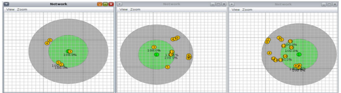
FIGURE 13. Random motes placement scenario for SLCPs framework process on Cooja architecture of grid consisting of 5, 10 and 15 CoAP motes and 1 RPL border router in each.
