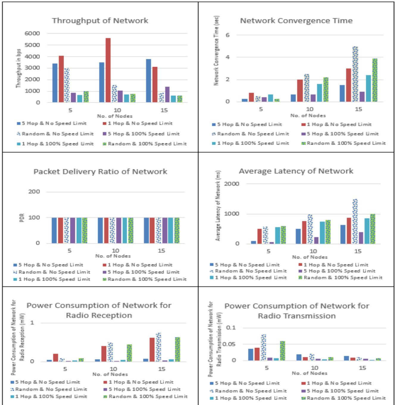
FIGURE 20. Overall results of performance evaluation parameters in terms 5hops, 1hop and random placement of nodes for no speed limit and 100% speed limit constraint scenarios of SLCPs framework.
