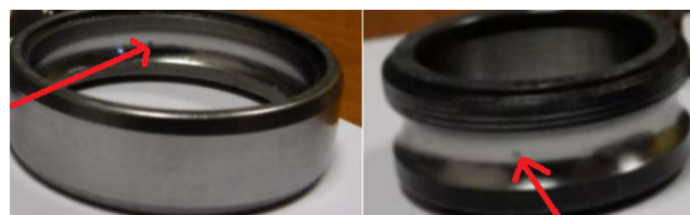
FIGURE 3. Artificial faults inflicted on the bearing parts with a laser beam.
