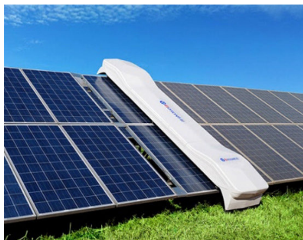
FIGURE 7. Boson robotic panel cleaning system [78].
