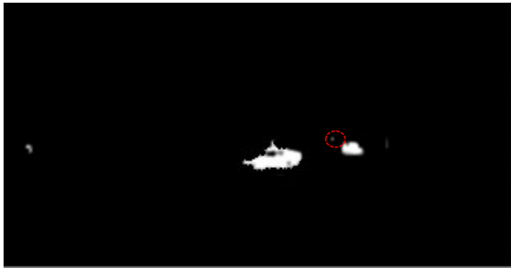
FIGURE 9. Results of the morphology operation process.
