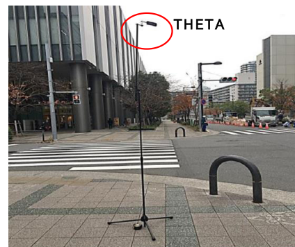
FIGURE 15. Theta camera installation at an intersection corner.
