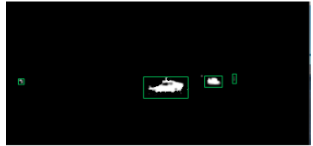
FIGURE 11. Moving objects detected in an image resulting from the morphology operation.
