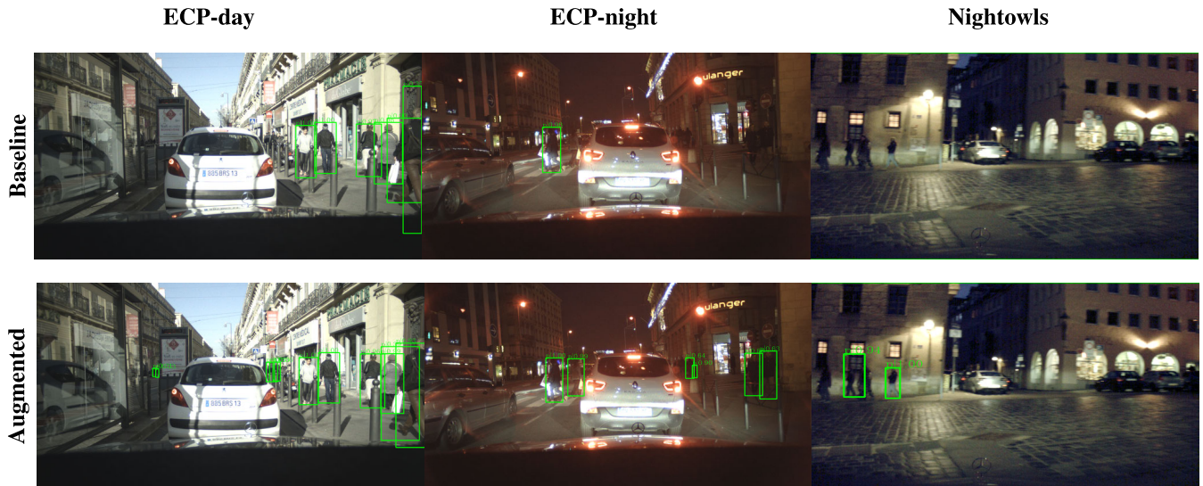
FIGURE 5. Detection samples for baseline and augmented model. The augmented model is more accurate on the night-time images, however some pedestrians are still not detected.
