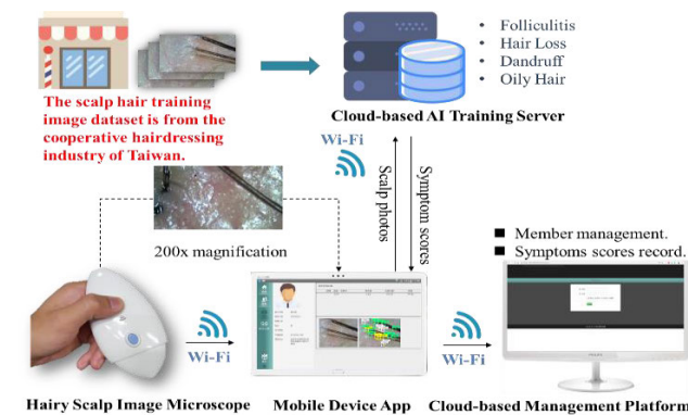
FIGURE 1. Architecture of the proposed ScalpEye system.
