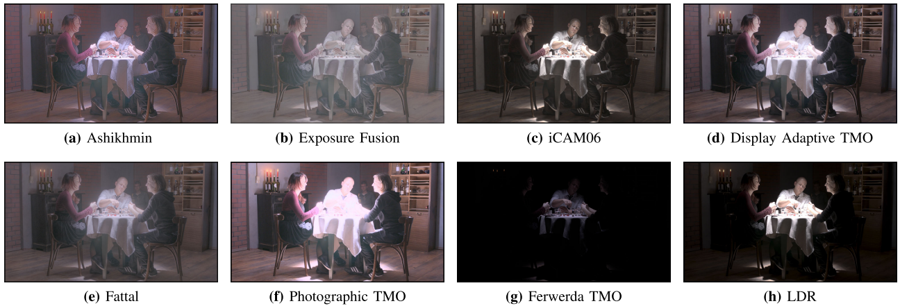
FIGURE 1. Visual representation of seven HDR to LDR mapping techniques along with an LDR representation.
