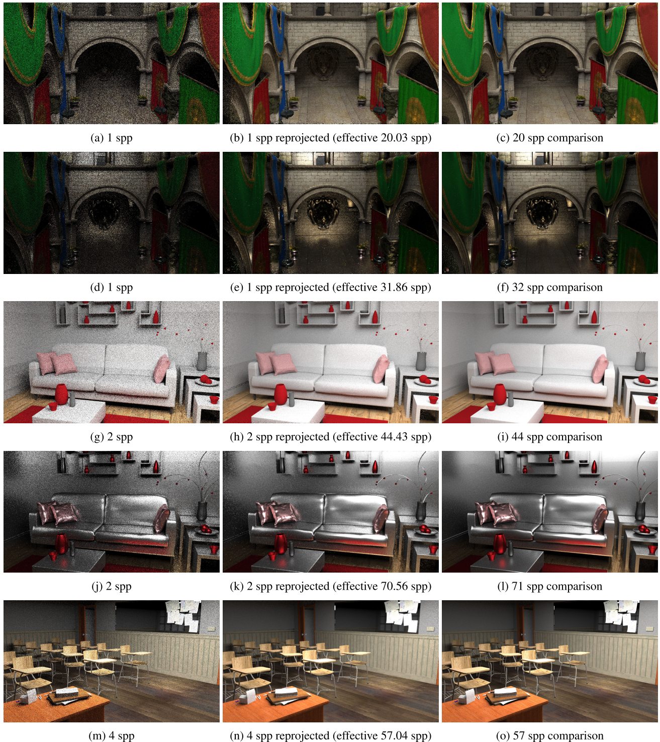
FIGURE 7. Frame comparison for the results in Section IV-B. Left column: left-eye frame with purely path traced n spp. Middle column: same left-eye frame obtained by spatiotemporally reprojecting the corresponding n spp right-eye frame onto an empty left eye and path tracing only the missing samples. Right column: purely path traced comparison frame with the spp count closely matching the effective spp of the reprojected frame.
