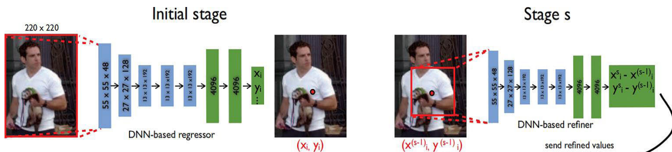
FIGURE 8. DeepPose’s DNN-based pose regressor and refiner.
