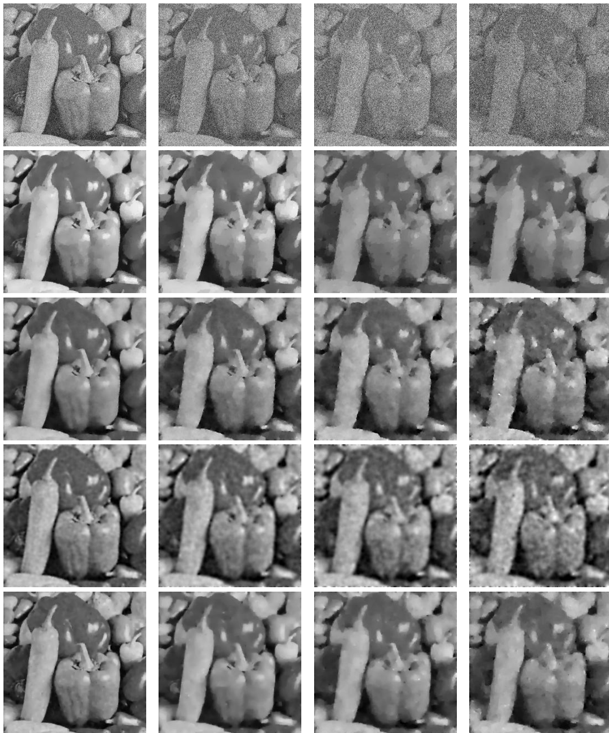
FIGURE 4. Restoration results obtained using the different methods. The results in the second to fifth rows were obtained using the TV model [20], SOHPDE model [29], FOHPDE model [30], and the proposed HPDEDD model, respectively.
