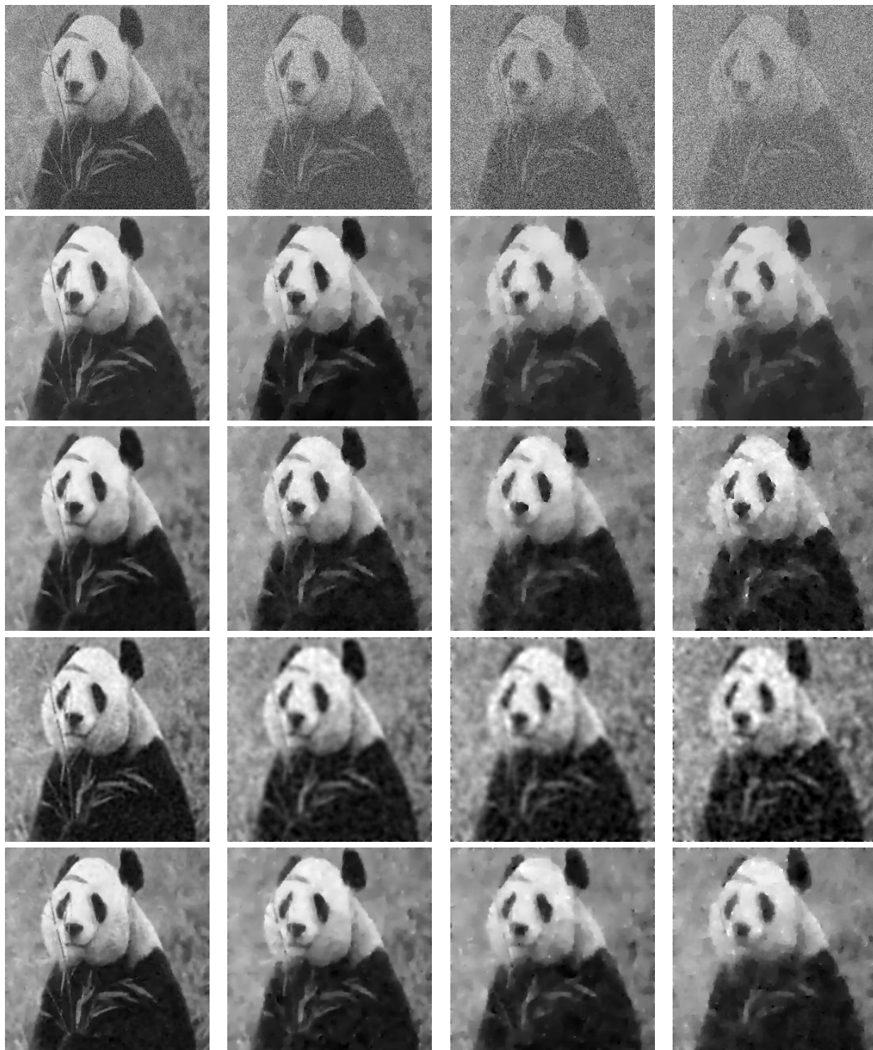
FIGURE 6. Restoration results obtained using the different methods. The results in the second to fifth rows were obtained using the TV model [20], SOHPDE model [29], FOHPDE model [30], and the proposed HPDEDD model, respectively.
