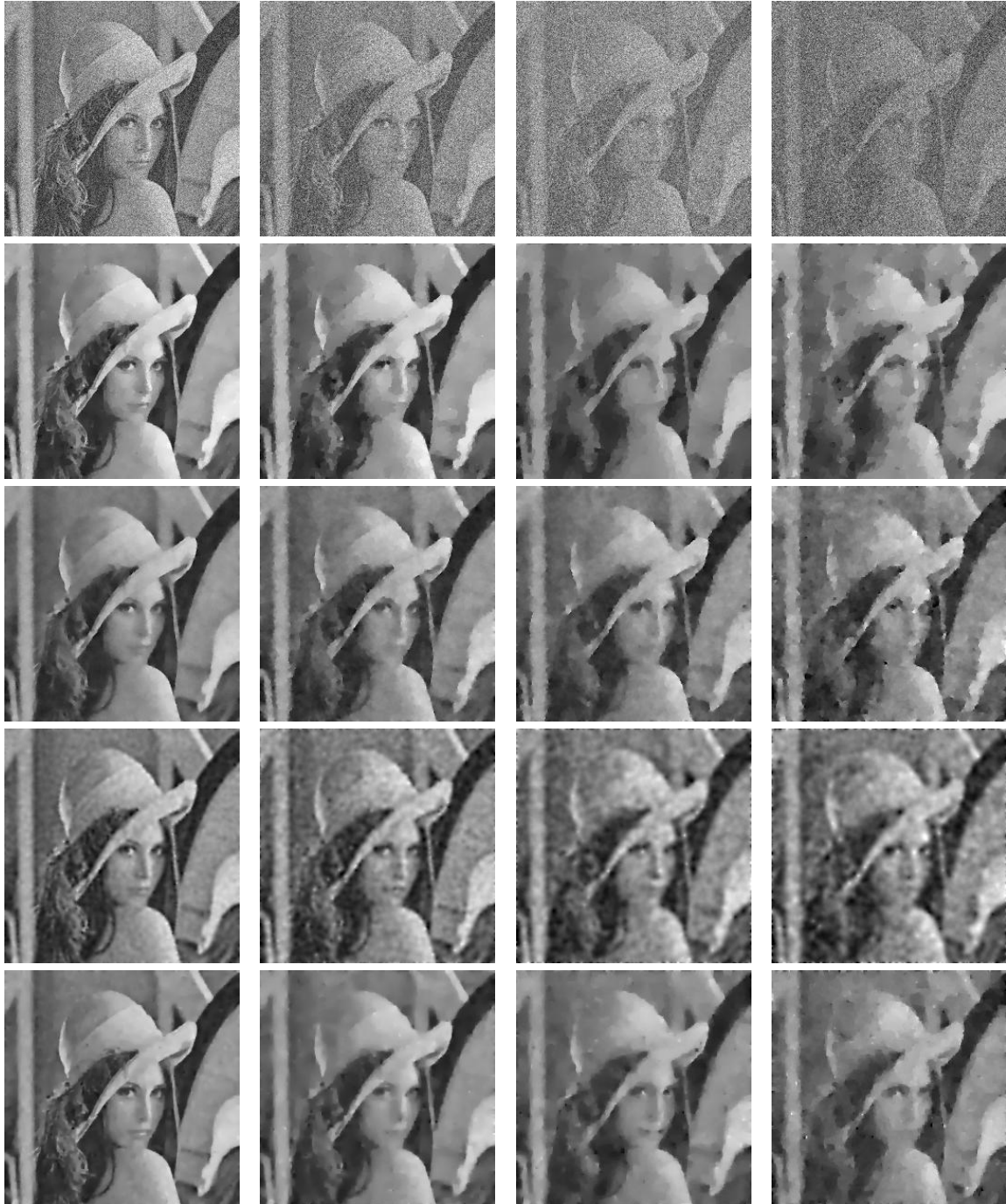
FIGURE 2. Restoration results obtained using the different methods. The results in the second to fifth rows were obtained using the TV model [20], SOHPDE model [29], FOHPDE model [30], and the proposed model, respectively.
