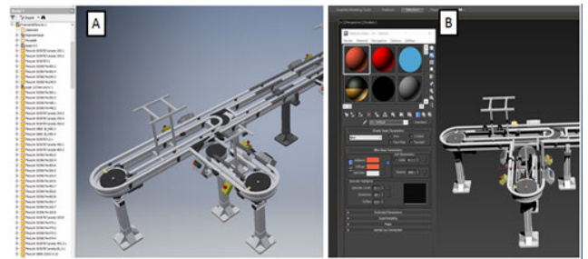
FIGURE 5. Digitization of the production line A-CAD model, B-graphic processing.
