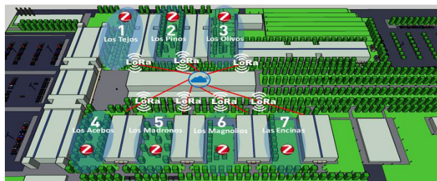
FIGURE 10. Schematic view of the simulation scenario implemented to analyze the campus botanical monitoring system, in which each one of the LoRaWAN/ZigBee sub-networks is presented.
