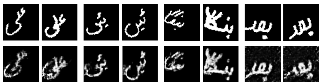
FIGURE 7. Rotated ligatures and its original counterpart. The samples in the first row are rotated ligature images (input y ), and the samples in the second row are the generated ligatures \hat{x} = F(y) .
