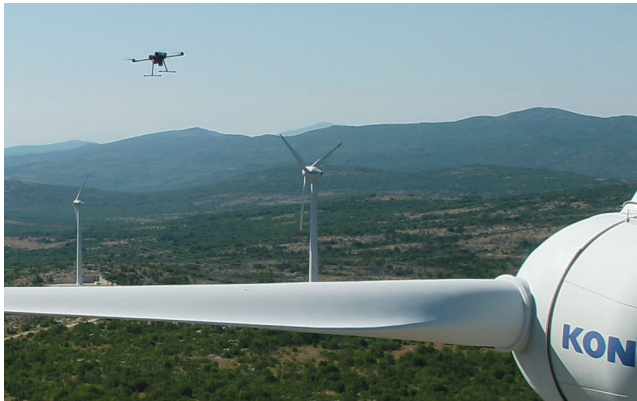
FIGURE 1. Custom built UAV equipped with a Velodyne VLP-16 LiDAR sensor filmed mid-flight while performing a manually operated inspection procedure on a wind-turbine blade.
