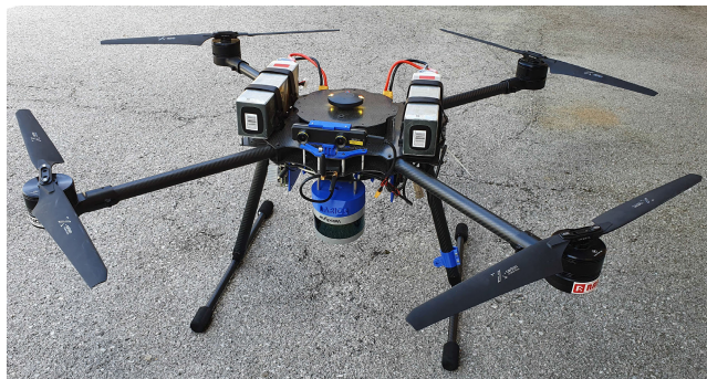
FIGURE 7. A custom-built LiDAR-equipped UAV used for performing wind-turbine blade inspection tasks.
