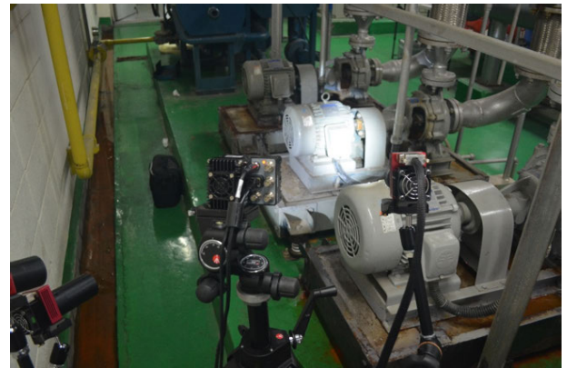
FIGURE 4. Water pump and camera setting.
