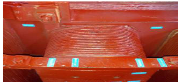
(c) Some temperature test paper on the pole surface(pole end region)
