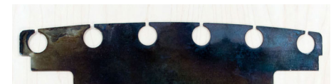
(e)Bluish traces due to overheating on the pole lamination in the upstream region
