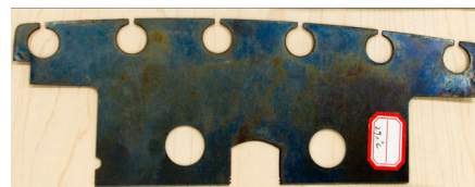
FIGURE 3. Bluish mark is shown on the pole lamination when heated to 290 °C in the oven.
