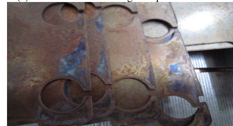
(d)Bluish traces due to overheating on the pole lamination in the downstream region
