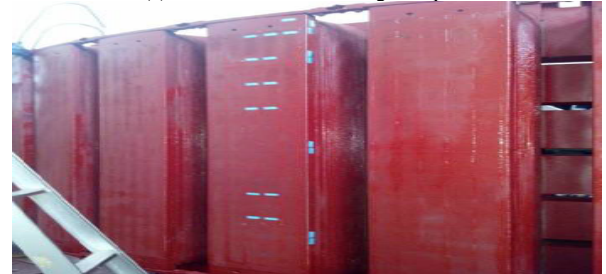
(b) Some temperature test paper on the pole surface(pole shoe)
