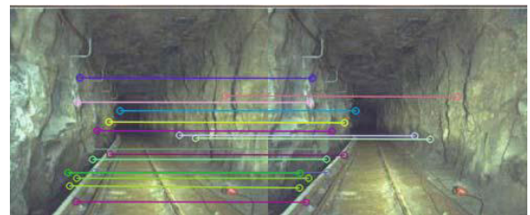
FIGURE 14. Stereo matching effect for a roadway image [66].
