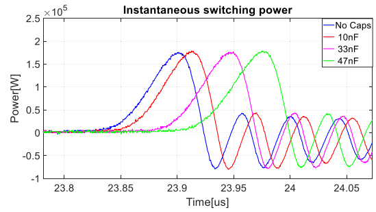
FIGURE 11. Switching power with gate-source capacitance.
