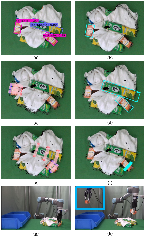
FIGURE 6. Entire procedure of picking rigid object. (a) Detection results. (b) Mapping 2D rotational bounding box to 3D for object with highest score. (c) Collision detection. The aims of (d) and (e) were the same as (b) and (c), respectively. (f) Obtaining feasible grasping pose. (g) and (h) represent the process of picking an object.
