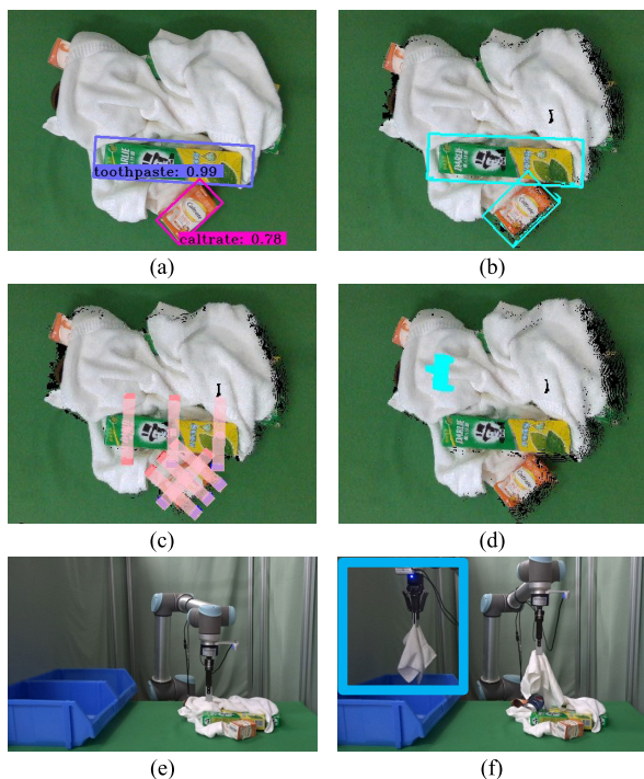
FIGURE 8. Entire procedure of picking towel. (a) Detection results. (b) Mapping 2D rotational bounding box to 3D for objects. (c) Collision detection. (d) Obtaining feasible grasping pose. (e) and (f) represent the process of picking a towel.
