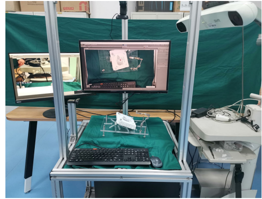
FIGURE 17. Augmented reality system error assessment platform.
