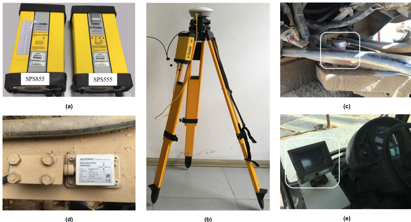
FIGURE 10. Experimental devices equipped on the SSR260 road roller. (a) SPS855 and SPS555 Trimble GNSS receivers; (b) base station; (c) multi-turn angle encoder; (d) inclination sensor; (e) industrial personal computer.
