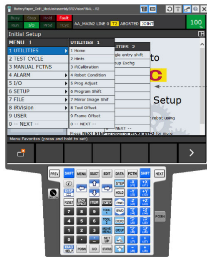
FIGURE 24. Off-Line robot programming environment menu.
