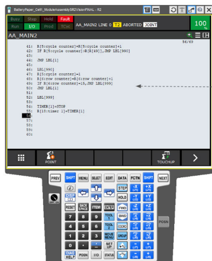
FIGURE 25. KAREL: ROBOGUIDE Off-line robot programming language.
