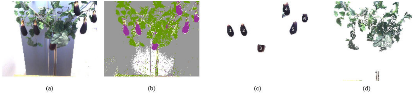
FIGURE 4. Segmentation process: (a) captured image; (b) classification of all the scene elements; (c) aubergine classification; (d) leaf classification.
