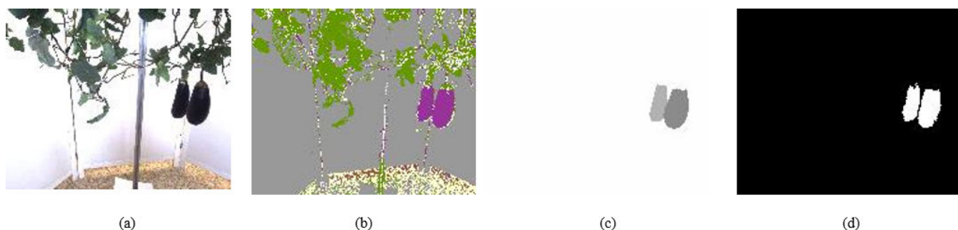
FIGURE 10. Experimental result - connected aubergine scene: (a) registered RGB image (b) pixel-based classification map (c) pixel labeling (d) output of the aubergine class.
