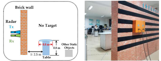
FIGURE 11. Geometry and photograph of radar data acquisition with no targets.
