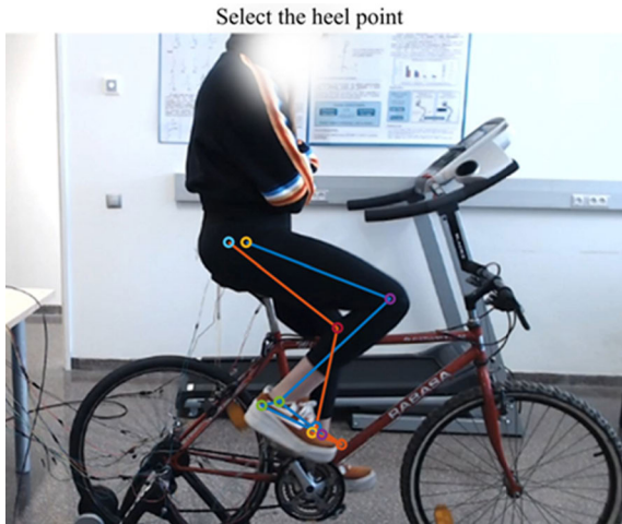
FIGURE 3. Example of the user interface at the first frame asking for the selection of key points of the leg that is on the same side of the webcam (heel point in this example).
