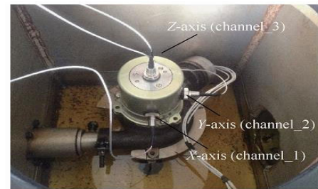
FIGURE 6. The installation of the airborne fuel pump test bench.
