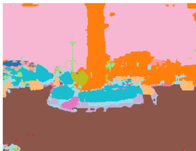
FIGURE 4. Color map corresponding to semantic segmentation of the image in Figure 3. Each color is mapped to a segmentation class (e.g. brown represents the “road” class).
