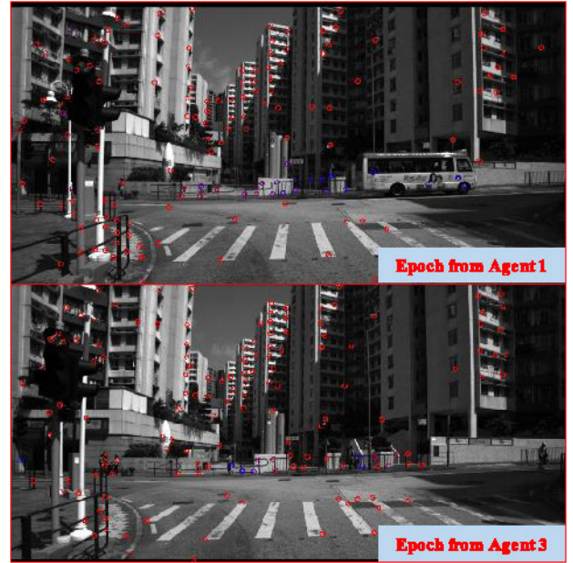
FIGURE 4. Illustration of overlapping area between agent 1 and 3 near an intersection. The red circles denote the detected features using the Shi [43] corner detection algorithm.
