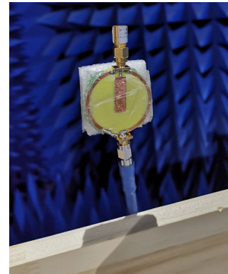
FIGURE 4. The antenna in microwave chamber for measurement.
