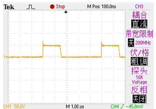
FIGURE 13. Terminal voltage of rectifier diode D1.
