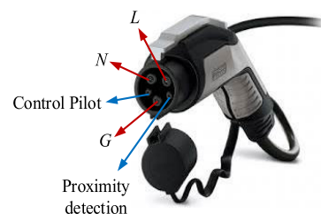
FIGURE 13. SAE J1772 charging connector of the V2V cable.
