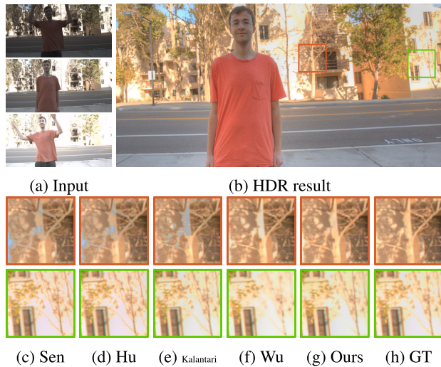
FIGURE 6. Comparisons of proposed and recent HDR imaging methods. (a) A set of input LDR images. (b) HDR result of our method. Magnification of red and green boxes by (c) Sen et al. [46], (d) Hu et al. [18], (e) Kalantari et al. [23], (f) Wu et al. [52], (g) our method, and (h) the ground truth.
