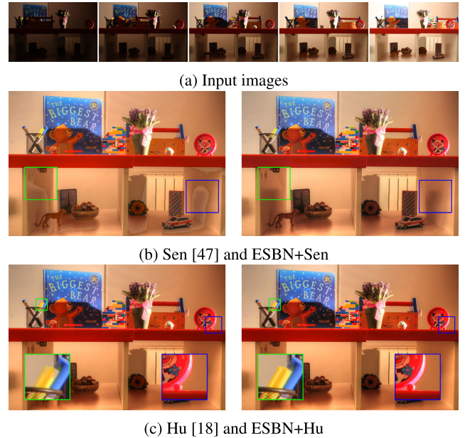
FIGURE 9. (a) An input image set with N = 5 by courtesy of Karadzovic-Hadziabdic [25]. (b) (c) Comparisons of the HDR results by the original and the modified version of the state-of-the-art methods.
